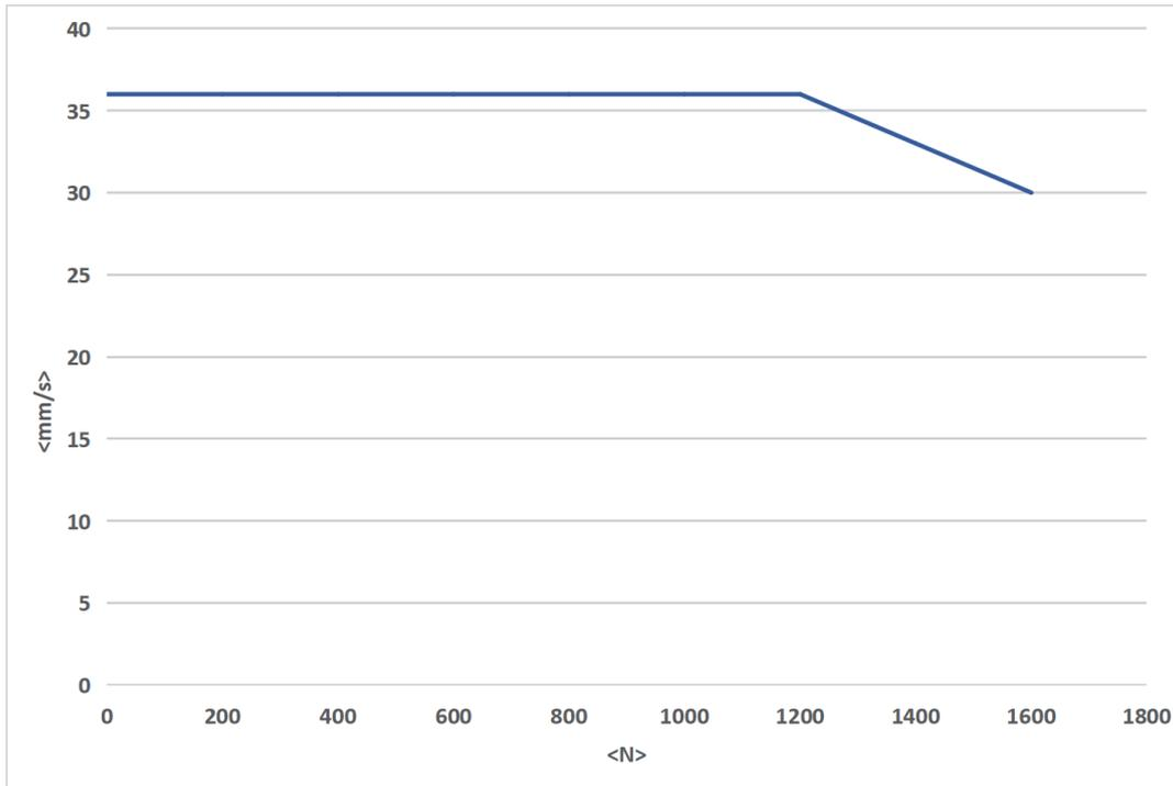
\*The curves above apply to a centrally placed load. With moment load, there will be increased friction in the columns, which will reduce the lifting force correspondingly.
